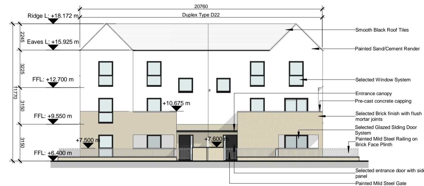
6 Duplex Block A South (Rear) Elevation 1 : 200
